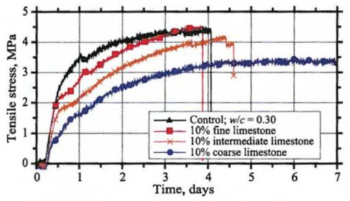
Figure 2.2 Restrained shrinkage results (Bentz et al. 2009b, quoting data from Bucher 2009) showing improved time to cracking results for low water-to-cement ratio concretes made cements with 10% limestone (and control without limestone). The coarse limestone exhibited much longer time to cracking.
