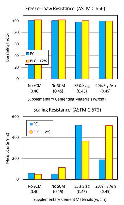
Figure 4.9 Results of freeze-thaw (top) and deicer-salt scaling tests for PC and PLC concretes with and without SCM (Thomas et al. 2010b).
