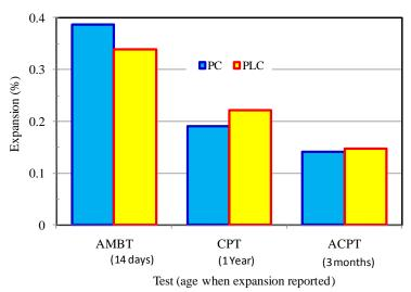
Figure 4.14 Expansion of mortar and concrete containing an alkali-silica reactive aggregate (Thomas et al. 2010b).
