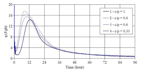
Figure 3.4 Heat production rate for mixtures with a CEM I 52.5 cement and high limestone contents at 20°C. "c/p" refers to the cement/powder (cement+limestone) ratio (Poppe and De Schutter 2005).
