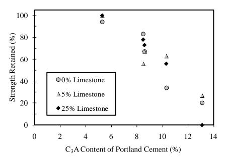
Figure 4.10 Strength retained after 2 years in MgSO<sub>4</sub> (1.5% SO<sub>3</sub>) solution (Matthews 1994).
