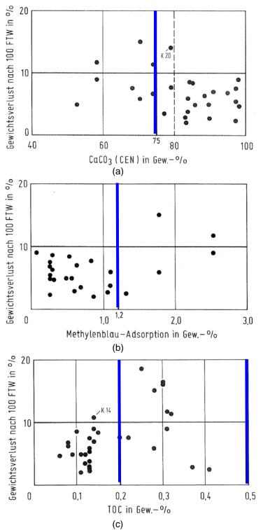
Figure 5.1 Freeze-thaw performance of non-air-entrained concretes made using cements with multiple limestone sources with a range of (a)  $CaCO_3$  contents, (b) MBI values, and (c) TOC contents. Vertical axis is weight loss after 100 freeze-thaw cycles. Horizontal line at 10% is the maximum limit selected for classifying acceptable concrete performance. Heavy blue lines are limits in EN197 (Note: EN197-1 has limits on TOC of 0.2% for -LL and 0.5% for -L). Source: Siebel and Sprung (1991).
