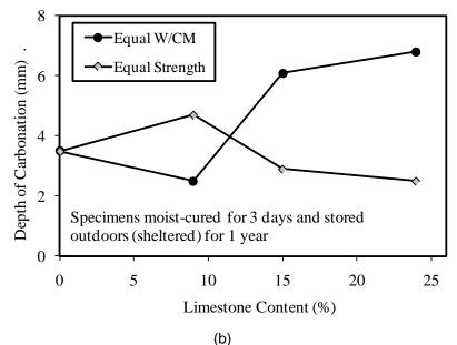
Figure 4.7 Effect of the limestone content of PLC on the carbonation of concrete mixes produced at equal w/cm or equal 28-day strength for specimens cured (a) 1 day or (b) 3 days (Barker and Matthews 1994).
