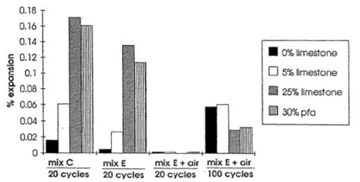
Figure 4.8 Effect of air entrainment on the freeze-thaw resistance of PC and PLC concrete (Matthews 1994).
