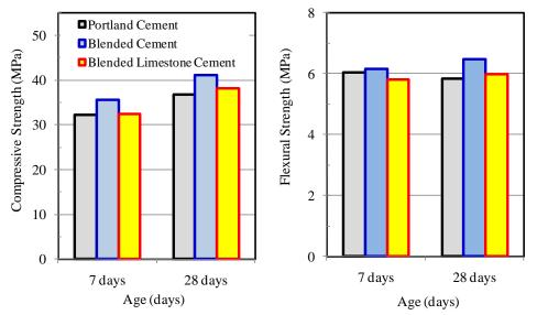
Figure 4.4 Strength data for concretes produced with different cements from the same plant (Thomas et al. 2010d).
