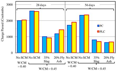
Figure 4.6 "Rapid Chloride Permeability Test" (ASTM C1202) data for PC and PLC concrete with and without SCM (Thomas et al. 2010b).
