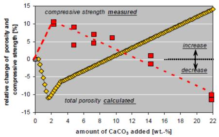
Figure 2.4 A correlation between porosity and strength development with limestone (Matschei et al. 2007b).
