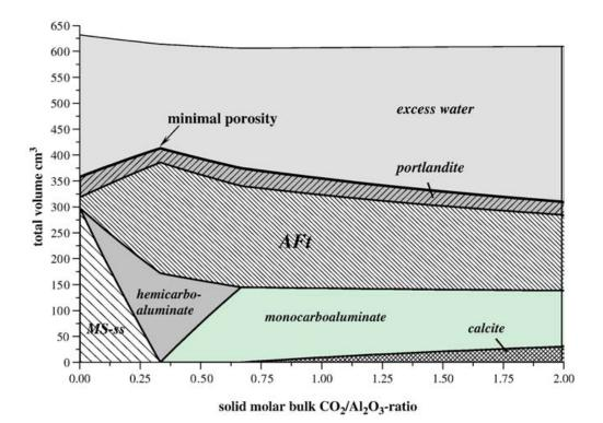
Figure 2.3 Calculated volumes of hydrate phases for a model mixture consisting of  $C_3A$ , portlandite and with fixed sulfate ratio (SO<sub>3</sub>/Al<sub>2</sub>O<sub>3</sub>=1) as a function of carbonate ratio (CO<sub>3</sub>/Al<sub>2</sub>O<sub>3</sub>) at 25°C (constant total amount of solids,  $C_3A$ +CaSO<sub>4</sub>+CH+Cc=3.25 mol, reacted with 500 g water) (Matschei et al. 2007a).
