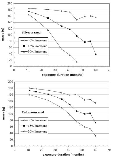
Figure 4.12 Change in mass of mortars with siliceous sand (top) or calcareous sand (bottom) stored in 1.8% MgSO₄ solution at 5°C (Skaropoulou et al. 2009a).
