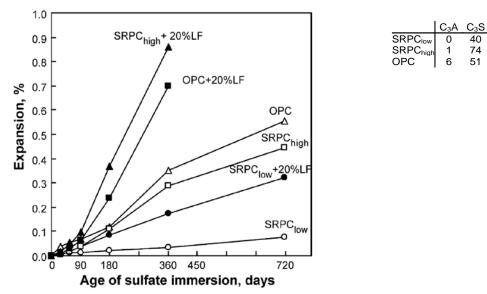
Figure 4.11 Effect of limestone on the expansion of mortars stored in  $5\% \text{ Na}_2\text{SO}_4$  (Irassar et al. 2005).
