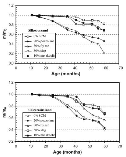
Figure 4.13 Relative mass change of mortars with siliceous sand (top) or calcareous sand (bottom) and SCM stored in 1.8% MgSO<sub>4</sub> solution at  $5^{\circ}$ C (Skaropoulou et al. 2009b).
