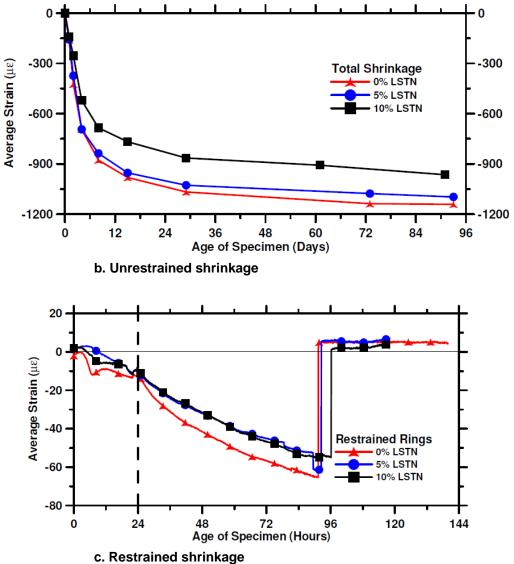
Figure 4.5 (a) Autogenous, (b) unrestrained, and (c) restrained shrinkage (ASTM C1581) for cements with no limestone, 5% and 10% limestone (Bucher et al. 2008).
