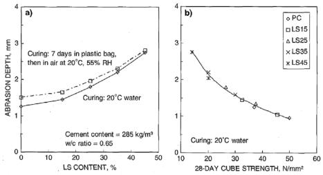
Figure 4.15 Effect of the limestone (LS) content of portland-limestone cement on the abrasion resistance of concrete (Dhir et al. 2007).
