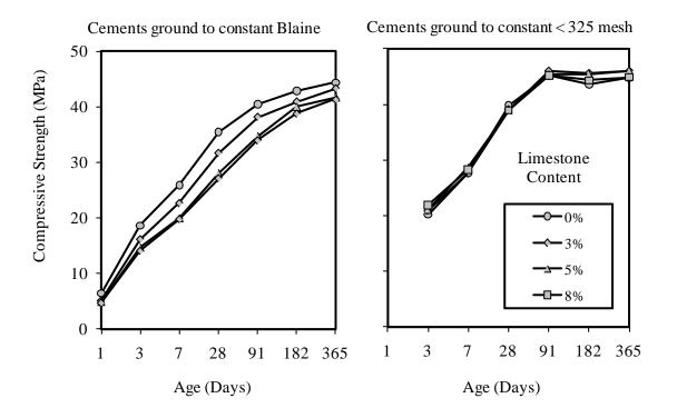
Figure 4.1 Strength development of mortars produced with PC and PLC ground to constant Blaine fineness (left) or constant Sub-325 Mesh (right) (Hawkins et al. 2005).
