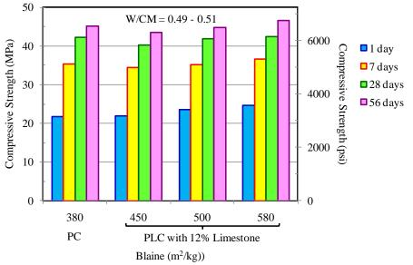
Figure 4.3 Effect of surface area (Blaine) on the strength of concrete (w/cm = 0.49 to 0.51) produced with PLC and PC from the same cement plant (Thomas et al. 2010b).
