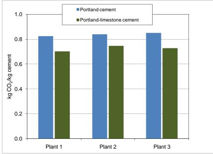
Figure 1.2 Specific CO<sub>2</sub> emissions from the production of portland cement or portland-limestone cement for 3 German cement plants (adapted from Schmidt 1992).
