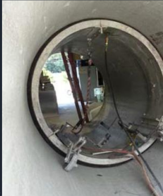
48" Pipe Deflected Joint Test Complete - No Leakage
