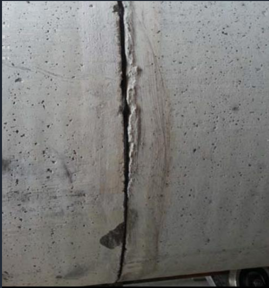
48" Pipe Deflected Joint Test Complete - No Leakage
