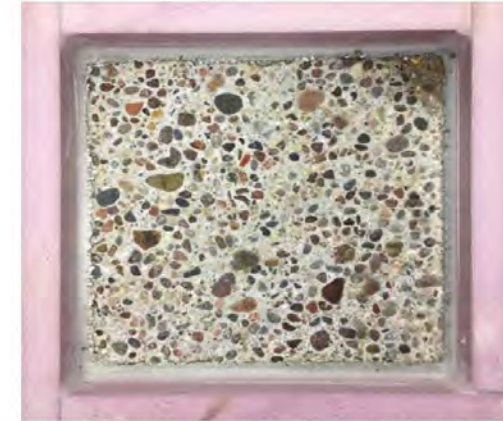
Figure 2. Control sample without waterproofing product and curing compound after 70 cycles of freezing and thawing
