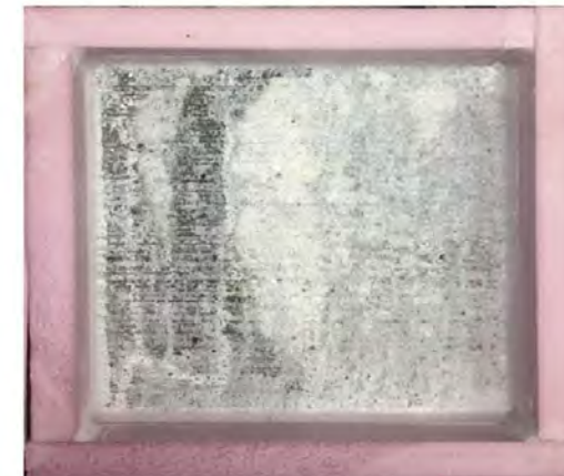
Figure 1. Sample with waterproofing product and curing compound after 70 cycles of freezing and thawing
