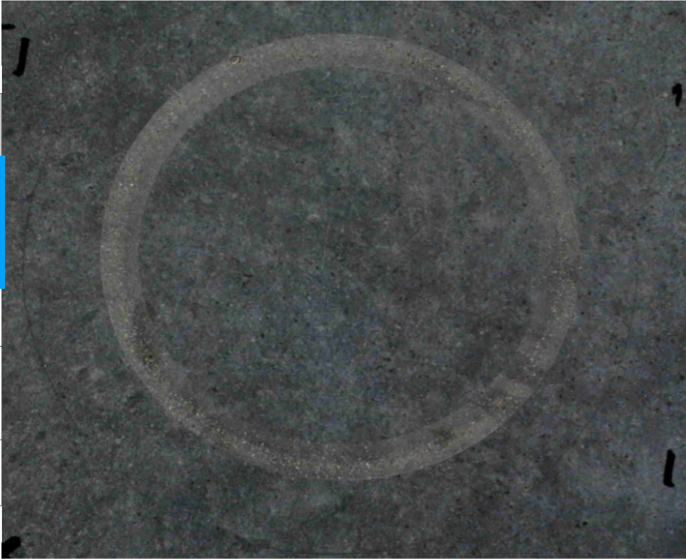
Wear ring from test 1 Mean depth 0.035 mm
