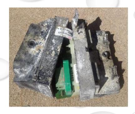
These enclosures are Cast Aluminum. The hydrochloric acid actually ate away the aluminum from the rubber seal between the two housing enclosures and allowed chemical and water into the circuitry.
